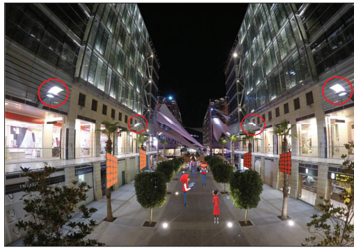
FIGURE 5. Walkway scenario in which the LED-based streetlights can be used as VLC APs, and RIS arrays can be installed on the palm trees to assist the wireless data transfer.
