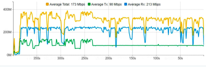
Fig. 7: Bandwidth test for the RF link with 80 MHz.
